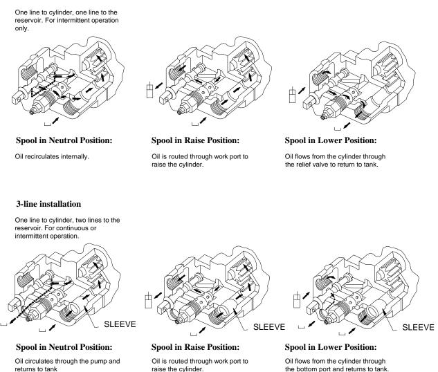
Note: Three line installation is recommended whenever possible by installing the sleeve supplied in the inlet port and connecting the optional return line to tank. This configuration maintains a lower operating temperature and a return line filter can be installed to filter return flow. Two line installations are for intermittent operation only.
